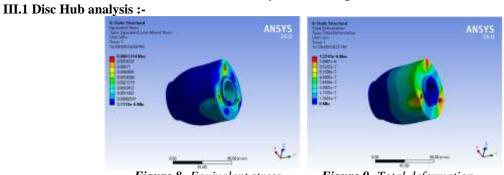
Figure 8- Equivalent stress
