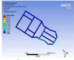
Figure 5- Equivalent stress
